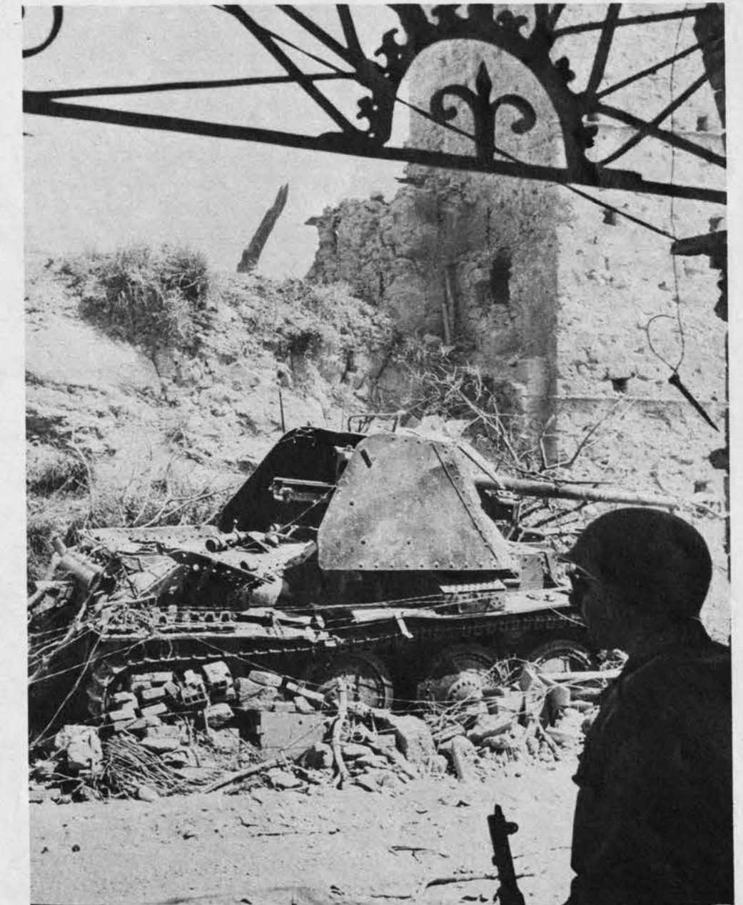
More familiar version of Nazi 75-mm. gun on the PzKw Czech chassis has cone-shaped gun housing set well forward. Czech suspension has short wheel base of four large bogies.
